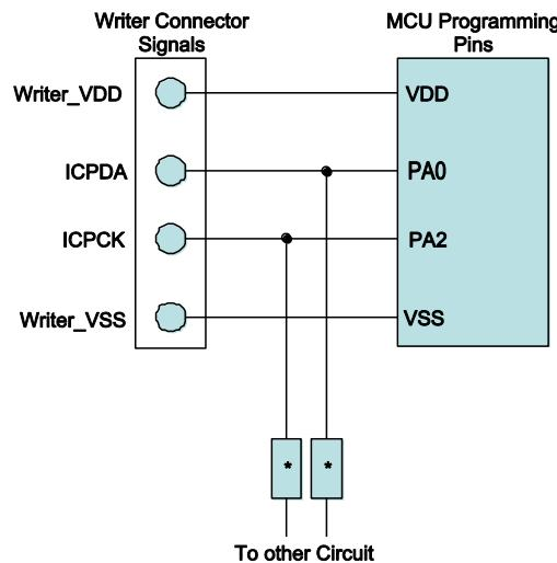
Note: \* may be resistor or capacitor. The resistance of \* must be greater than  $1k\Omega$  or the capacitance of \* must be less than  $1nF$ .
